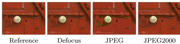
Fig. 1 Example of a reference image and three degraded images with blur or compression. The images are from the TID2008 dataset [23]
