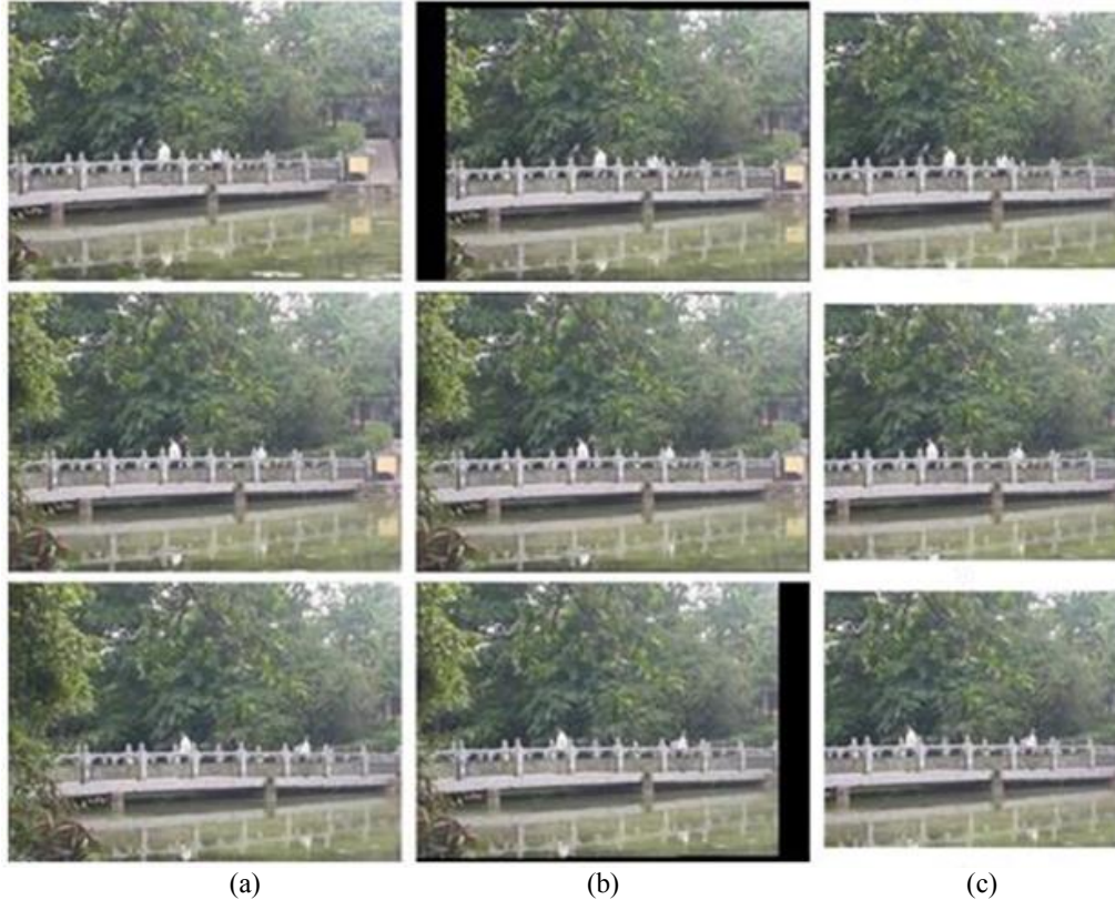
Figure 5. Image sequence preprocessing.(a) Input image sequence;(b) Match Image; (c) Extract common region
